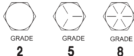
BOLT HEAD GRADE MARKING
